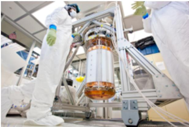
The LUX (Liquid Underground Xenon experiment), based in the Homestake mine in Lead South Dakota, looks for rare dark matter interactions with a sensitive, ultra cold detector. To avoid contamination from cosmic-rays and radioactivity, these massive machines must be placed deep underground in old mines.
